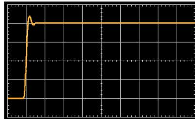
Figure 9. Step response with 3-pF feedback capacitance (20 ns/div).
