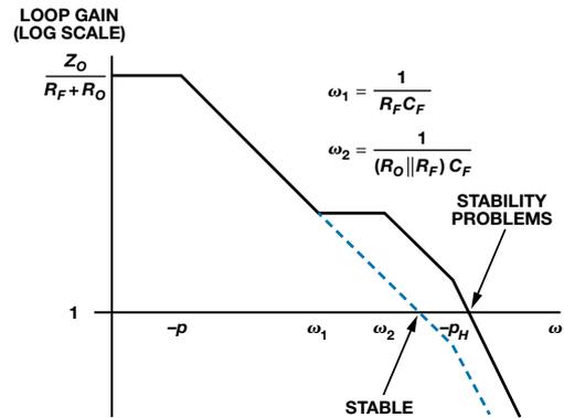
Figure 4. Bode plot of CFA-based TIA with feedback
