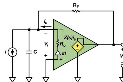
Figure 3. Practical CFA-based TIA including parasitic capacitance.
