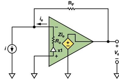
Figure 2. Practical CFA with unity-gain buffer used as a TIA.
