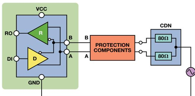
Figure 4. Coupling/decoupling network for a half-duplex RS-485 device.
