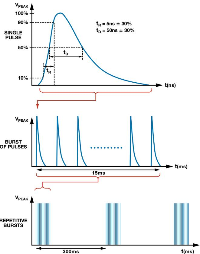
Figure 2. IEC 61000-4-4 EFT 50  $\Omega$  load waveforms.
