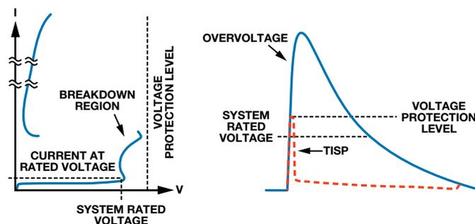
Figure 8. TISP switching characteristic and voltage limiting waveshape.
