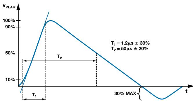
Figure 3. IEC 61000-4-5 surge 1.2/50  $\mu\text{s}$  waveform.
