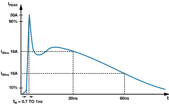
Figure 1. IEC 61000-4-2 ESD waveform (8 kV).
