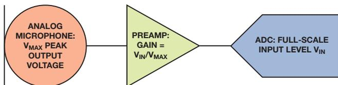
Figure 1. Analog microphone input signal chain with preamp to match microphone output level to ADC input level.
