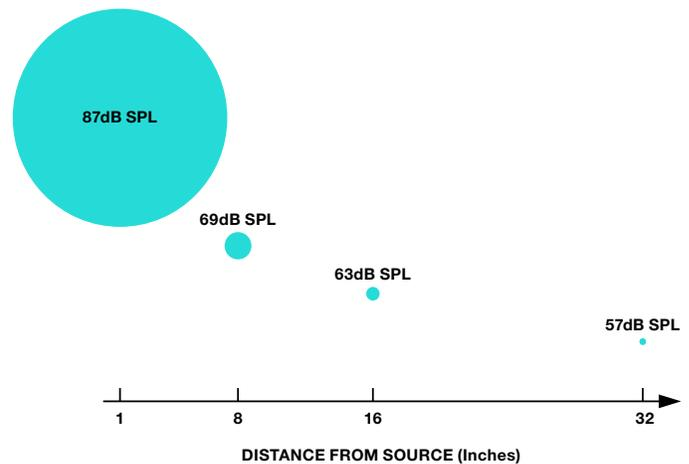
Figure 3. Sound pressure level at the microphone is reduced as the distance from the source increases.
