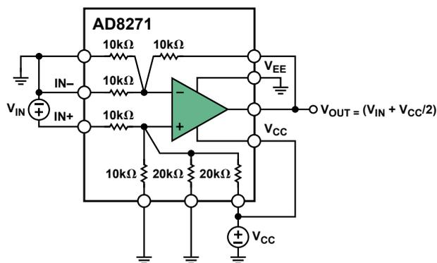
Figure 2. AD8271 shifts output to midsupply with no external components.
