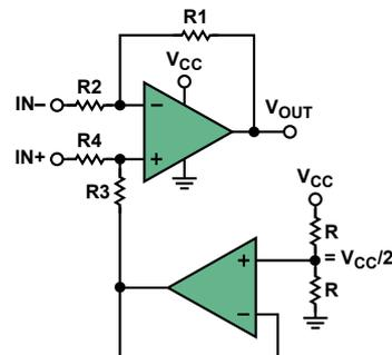
Figure 1. Single-supply difference amplifier with midsupply output.
