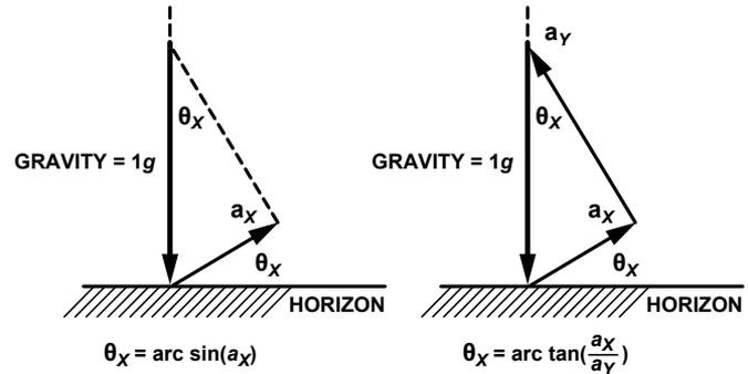
Figure 3. MEMS tilt sensor operation.
