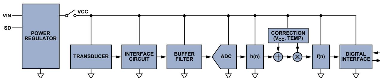
Figure 1. Example of a sensor system.
