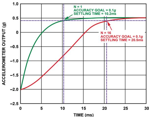
Figure 5. Power-on transient response.
