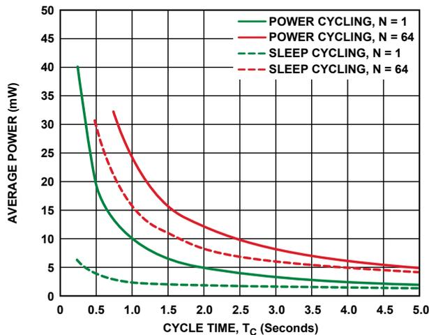
Figure 6. Cycle time vs. average power dissipation.
