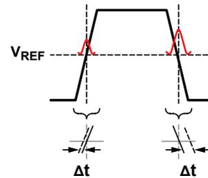
Figure 3. Jitter impact of reflected signal due to improper termination.
