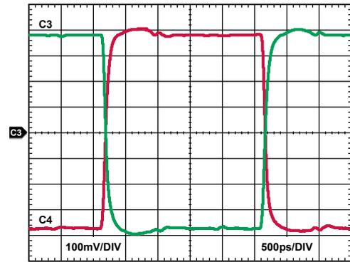
Figure 2. ADCLK954 clock buffer output waveforms with 3.3-V supply.
