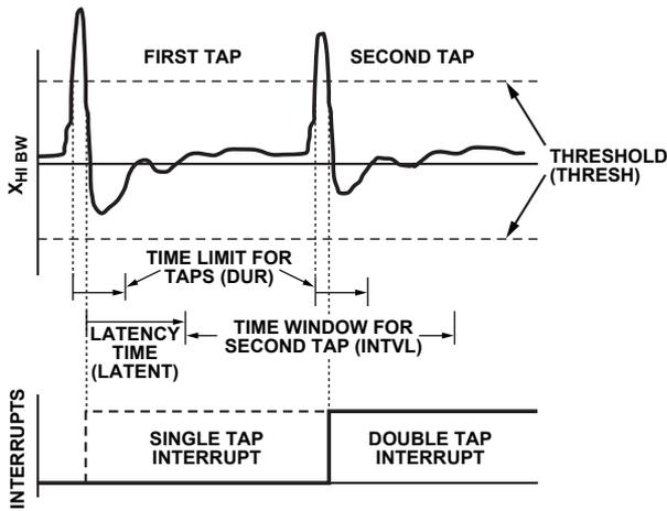
Figure 2. SINGLE\_TAP and DOUBLE\_TAP interrupts.
