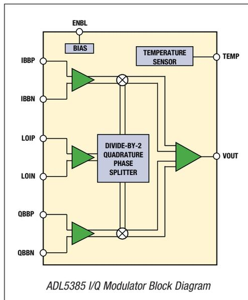
desired RF output. LO symmetry is also extremely important as it directly contributes to the sideband suppression.
