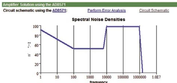
Figure 6. Typical noise spectrum for a photodiode application.
