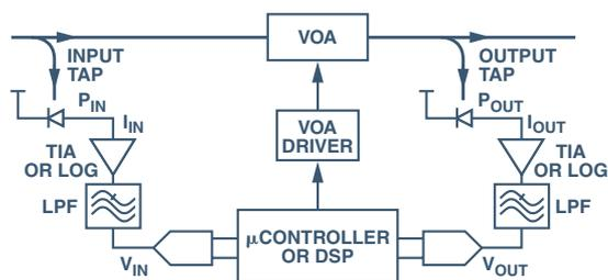
Figure 1. VOA adaptive control loop. Input and output optical taps are used to measure the attenuation of the VOA. The measured signal is compared to a desired setpoint level using an error integrator, implemented in software. The difference signal is used to control the attenuation of the VOA, yielding a closed-loop design.
