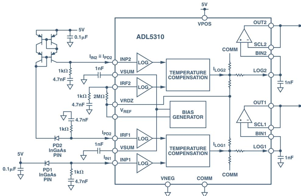
Figure 6. Alternative solution using a modified Wilson current mirror.
