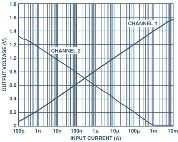
Figure 4. Transfer functions for the two outputs.
