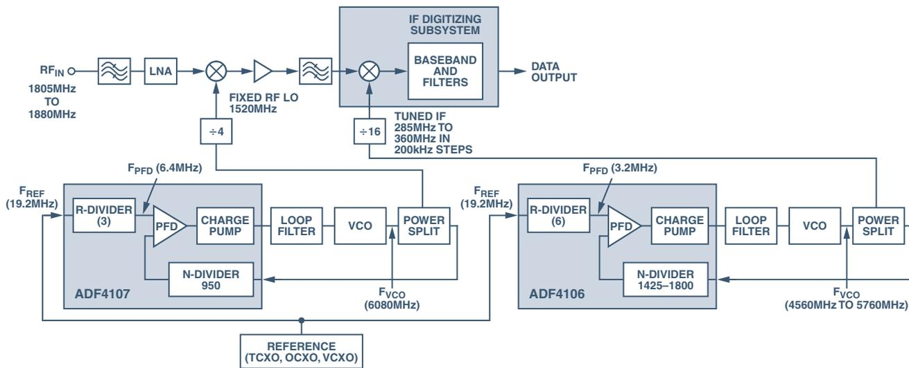
Figure 2. Alternative receiver block diagram
