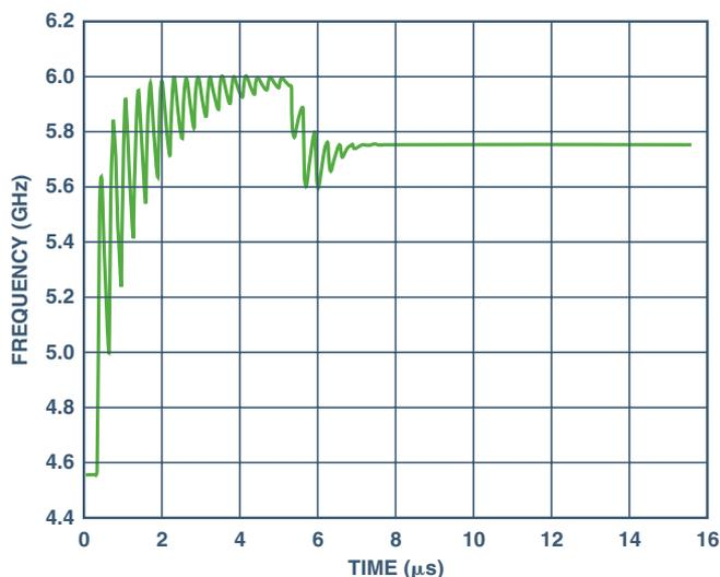
Figure 3. Lock time for the tuned IF.
