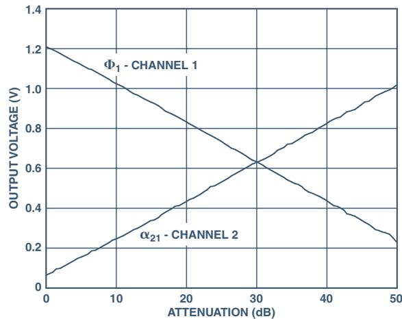
Figure 3. Transfer functions for the two outputs. Channel 1 provides the absolute output power, while Channel 2 provides the relative attenuation between the two channels.
