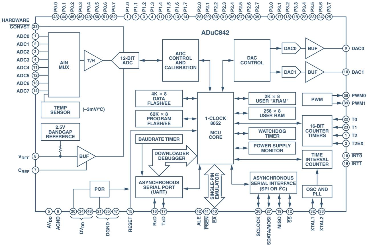
Figure 4. ADuC842 block diagram.
