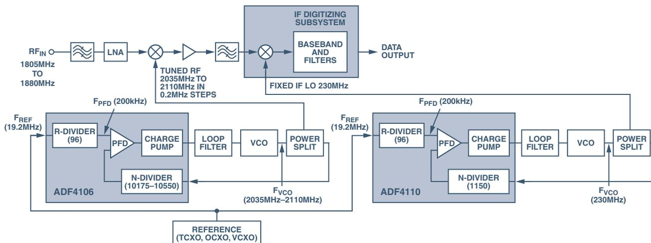
Figure 1. Block diagram of a traditional superheterodyne receiver.
