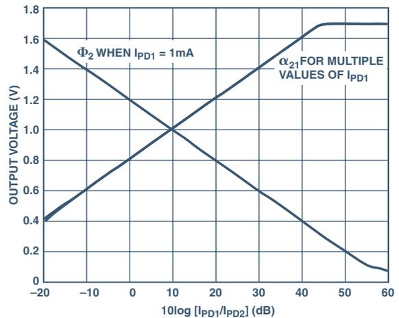
Figure 7. Absorbance and absolute power transfer functions for Wilson-mirror ADL5310 combination.
