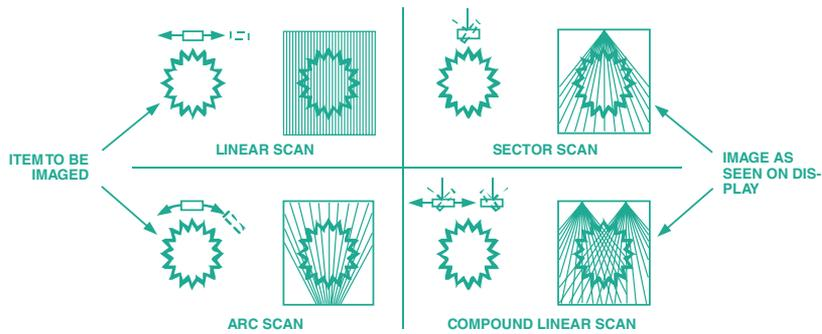
Figure 2. Single-transducer image generation.
