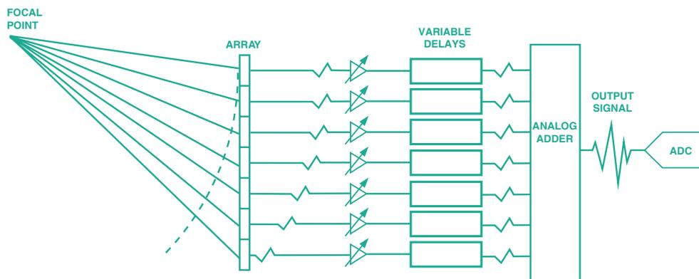
Figure 4. Simplified block diagram of ABF system.
