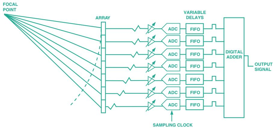
Figure 5. Simplified block diagram of DBF system.
