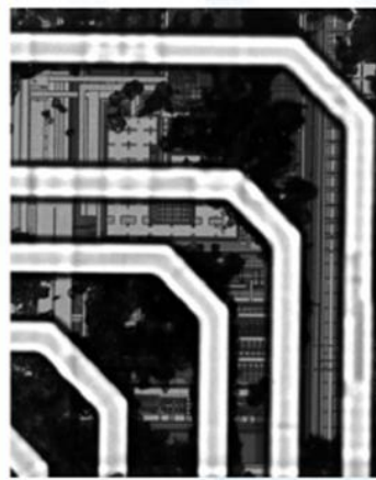
LEM result of the failing unit comparable with the results from a known good unit
