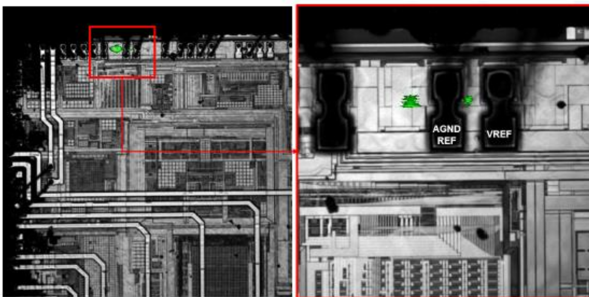
Figure 2. Image of the abnormal resistance-change or hotspot observed on the unit
