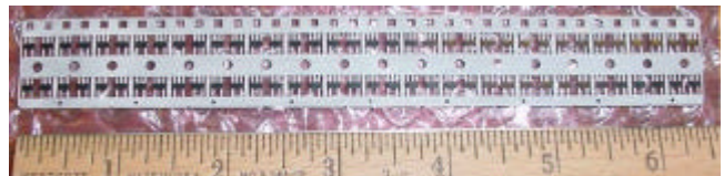
Figure 1a: 2 x 36 leadframe strip of 5-lead SOT packages.
