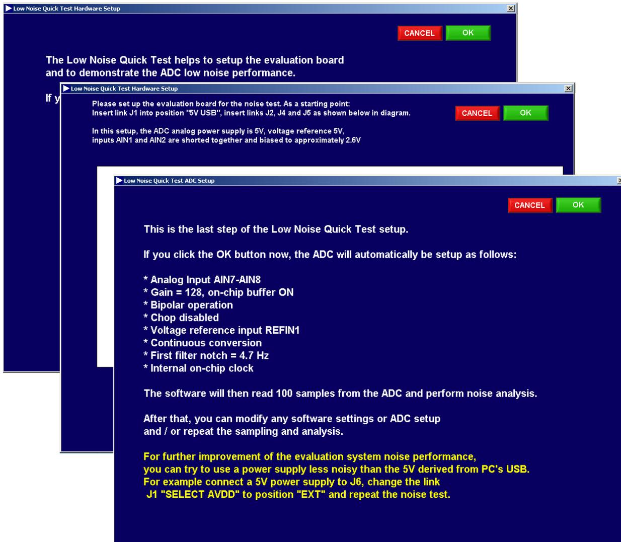
Figure 10. Low Noise Quick Test Hardware Setup
