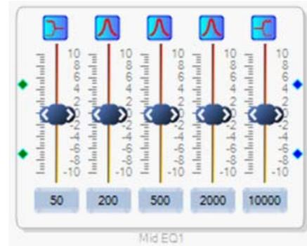
Figure 29. Configured 5-Band EQ Cell
