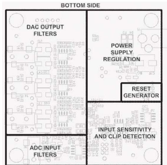
Figure 5. Board Layout Block Diagram (Bottom Side)
