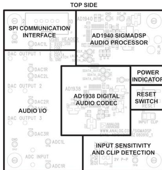
Figure 4. Board Layout Block Diagram (Top Side)
