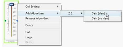
Figure 22. Adding a Channel to the Volume Control
