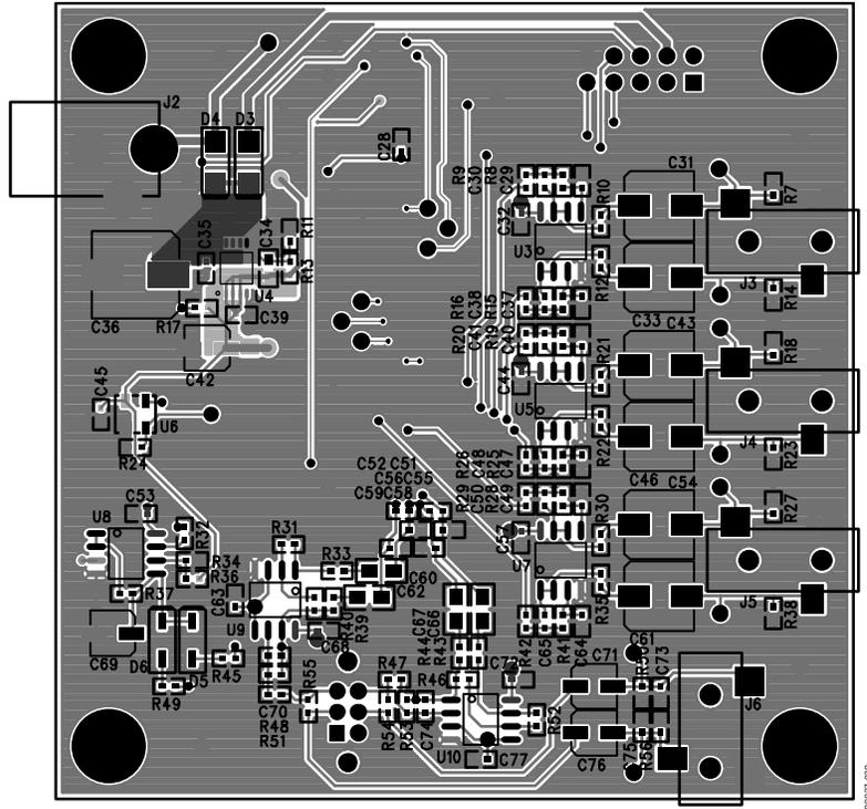
Figure 38. Board Layout, Page 3—Bottom Layout and Screen
