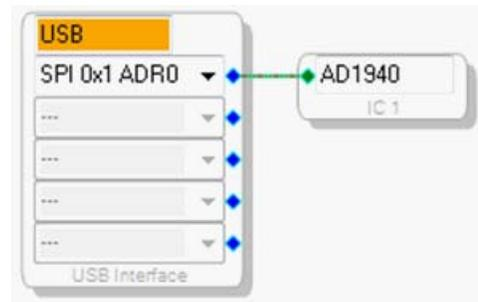
Figure 14. Connecting the USBi to an AD940 IC
