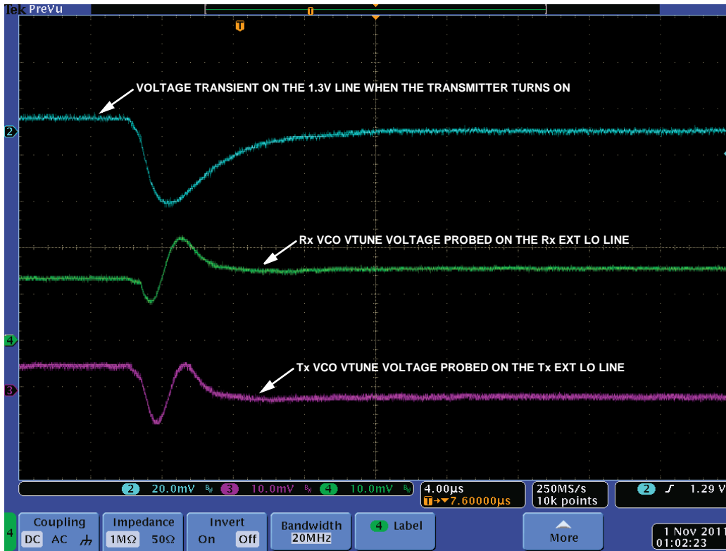
Figure 89. Voltage Transient on the 1.3 V Supply and Vtune of the Rx and the Tx VCO
