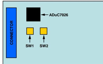
Figure 9. ISEB Switch Locations for Flashing the Microcontroller
