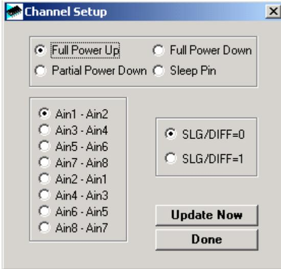
Figure 6. The Channel Setup Screen, Pseudo-differential configuration
