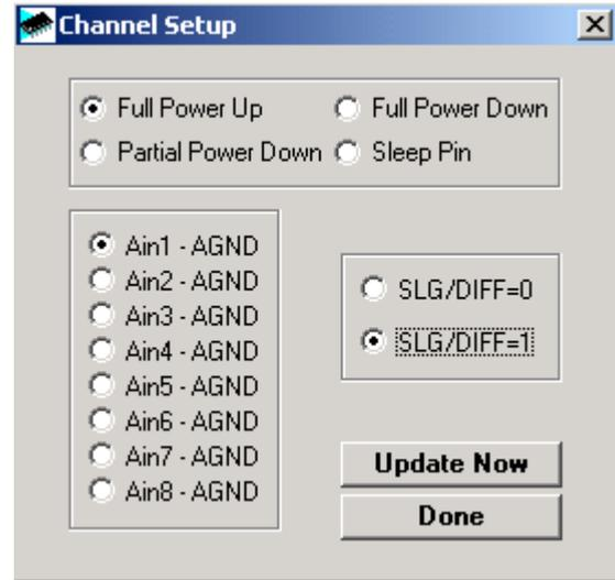
Figure 7. The Channel Setup Screen, Single Ended configuration
