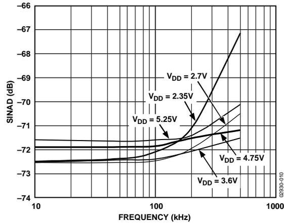
Figure 10. AD7476A SINAD vs. Input Frequency at 1 MSPS
