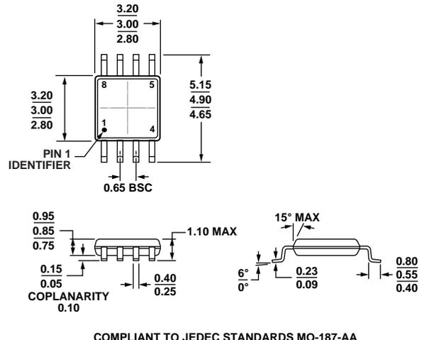
Figure 34. 8-Lead Mini Small Outline Package [MSOP] (RM-8)
