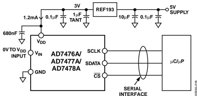
Figure 18. REF193 as Power Supply to AD7476A/AD7477A/AD7478A
