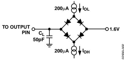
Figure 2. Load Circuit for Digital Output Timing Specifications
