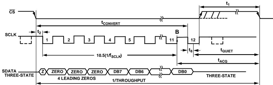
Figure 27. AD7478A in a 12 SCLK Cycle Serial Interface
