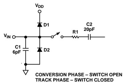
Figure 19. Equivalent Analog Input Circuit
