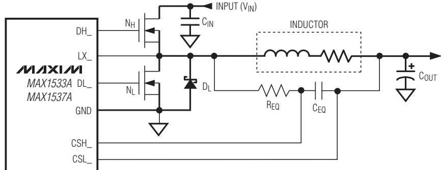
b) LOSSLESS INDUCTOR SENSING
