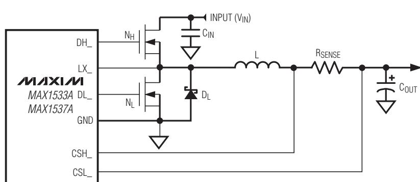
a) OUTPUT SERIES RESISTOR SENSING
