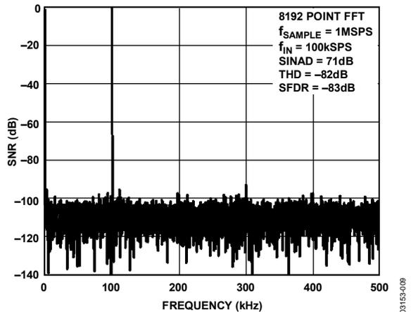
Figure 9. AD7451 Dynamic Performance for  $V_{DD} = 5 \text{ V}$
