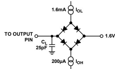
Figure 4. Load Circuit for Digital Output Timing Specifications
