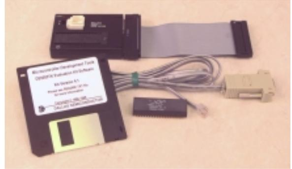
DS5000T for operation in the target system without detailed knowledge of the operation of the DS5000's bootstrap loader interface. The DS5000TK Evaluation Kit not only serves as a first-time evaluation system for the DS5000 or the DS5000T, but also performs the equivalent function of an EPROM programming system throughout the prototyping phase of the design cycle.
