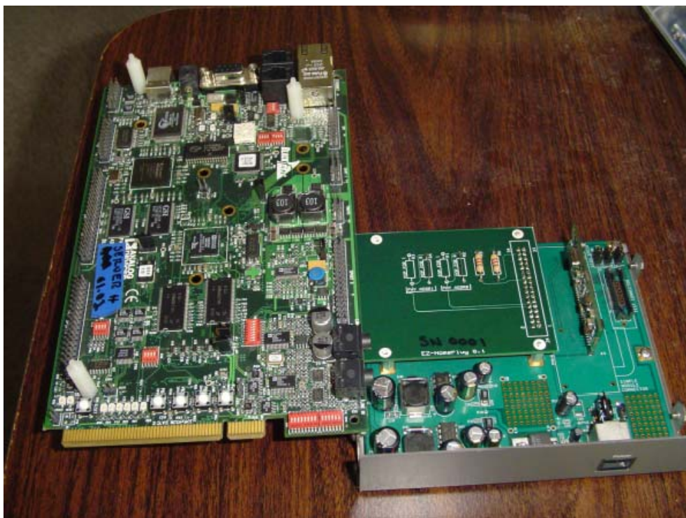
图3 ADSP-BF537 EZ-KIT Lite, EZ-HomePlug和EDK5200的组装
