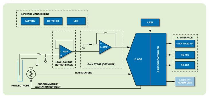
Note: The signal chains above are representative of the system block diagram of a system block diagram of pH meter design. The technical requirements of the blocks vary, but the products listed in the table below are representative of ADI's solutions that meet some of those requirements.
