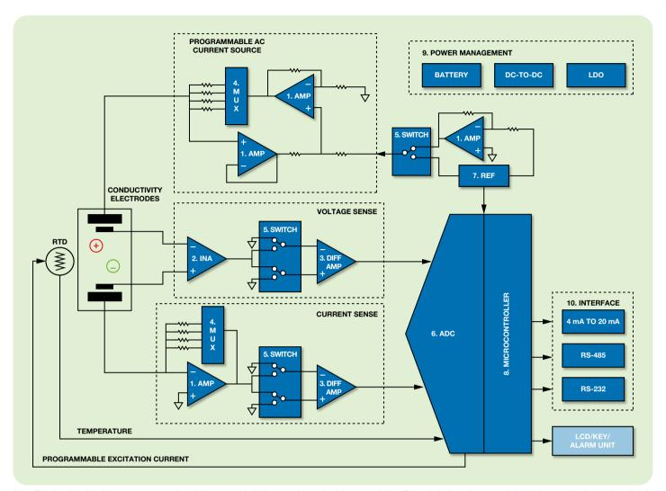
Note: The signal chains above are representative of the system block diagram of a conductivity meter design. The technical requirements of the blocks vary, but the products listed in the table below are representative of ADI's solutions that meet some of those requirements.
