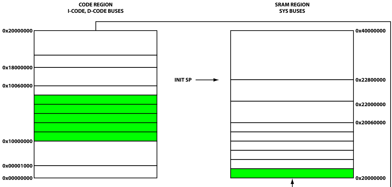
Figure 2-10: SRAM Code and SRAM Partitions for SRAM_CODE = 5
