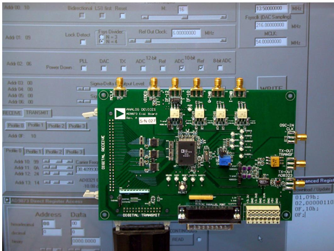
Figure 11. AD9873 evaluation board and software interface.
