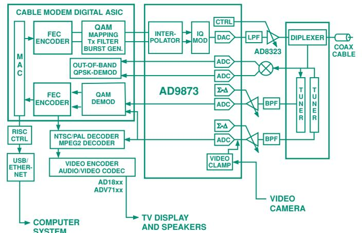
Figure 4. Intelligent system partitioning helps to solve the challenge of optimizing price, performance, size, and power in broadband modem designs.
