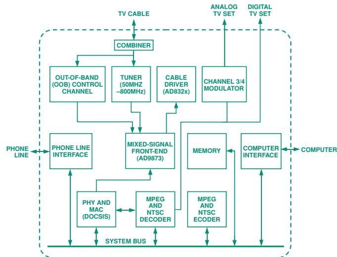
Figure 2. Inside a typical digital set-top box.
