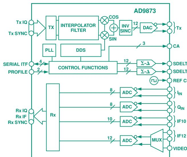
Figure 3. AD9873 functional block diagram.
