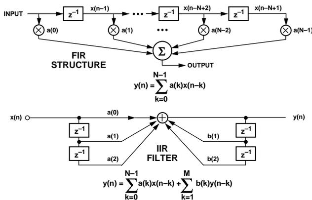
Figure 1. Filter equations and their delay-line models.
