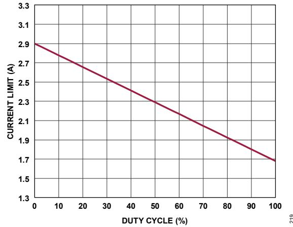
Figure 24. Top MOSFET Current Limit vs. Duty Cycle
