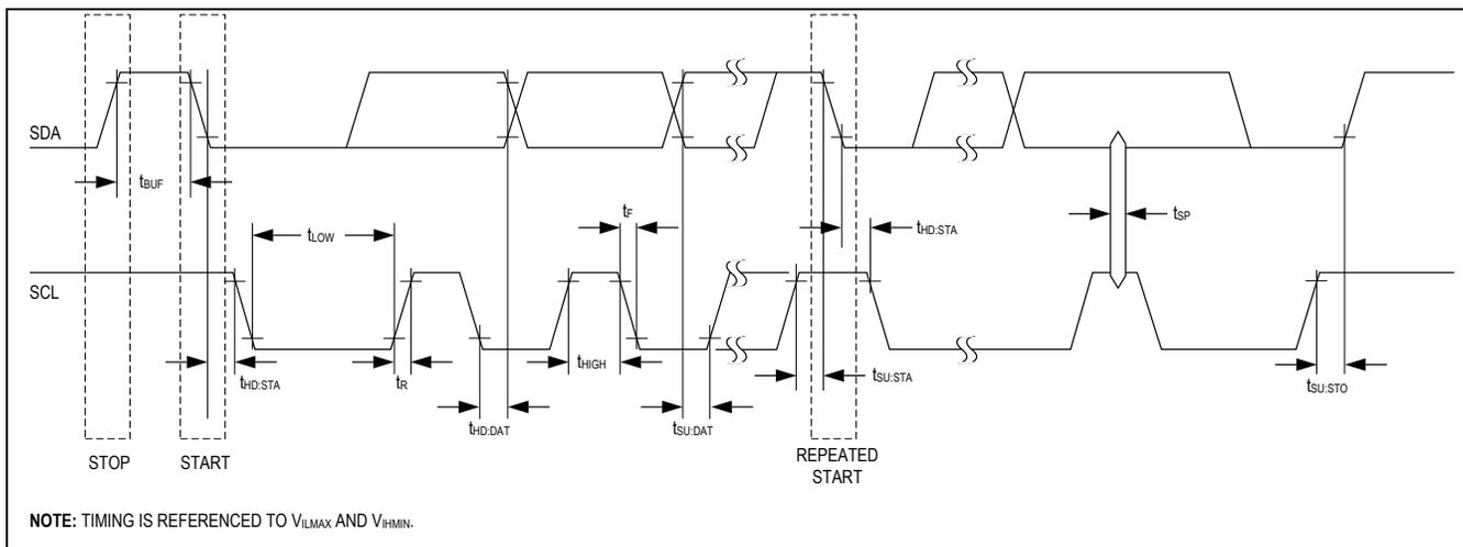
Figure 1. I<sup>2</sup>C Timing Diagram
