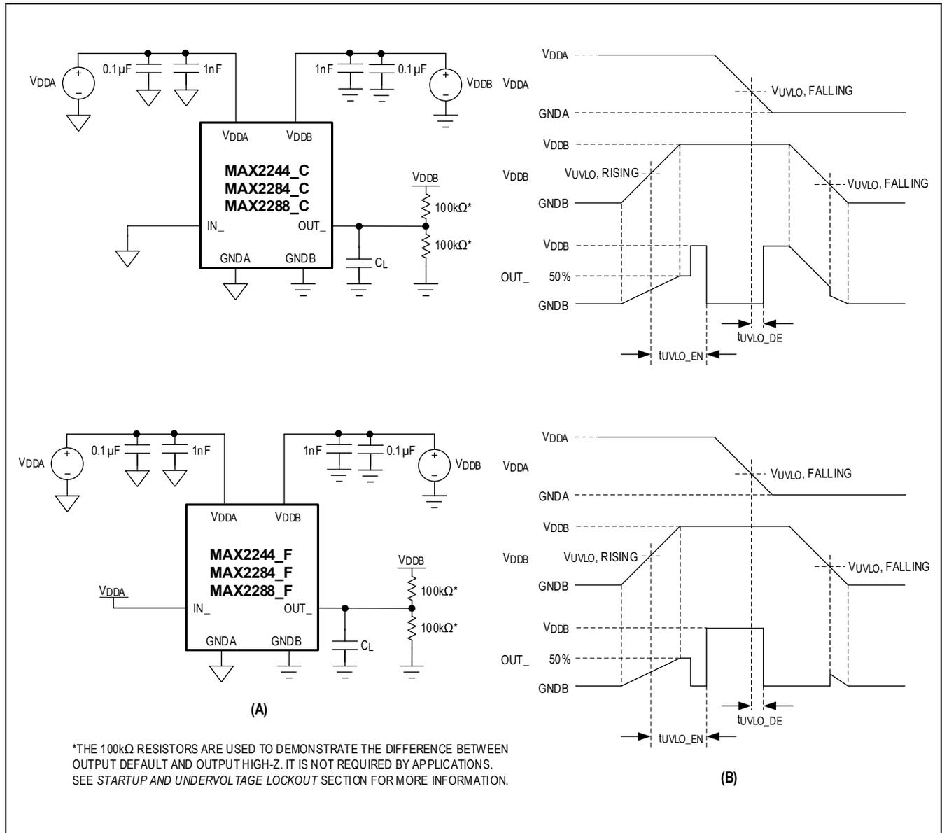
Figure 3. UVLO to Output Timing Diagrams ( $t_{UVLO\_EN}$ ,  $t_{UVLO\_DE}$ )
