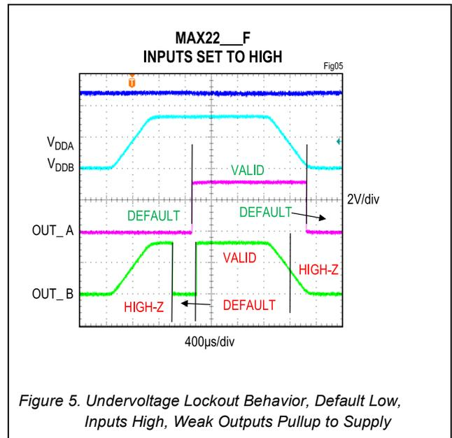
Figure 5. Undervoltage Lockout Behavior, Default Low, Inputs High, Weak Outputs Pullup to Supply
