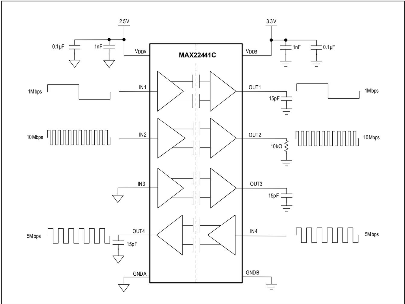
Figure 13. Example Circuit for Supply Current Calculation
