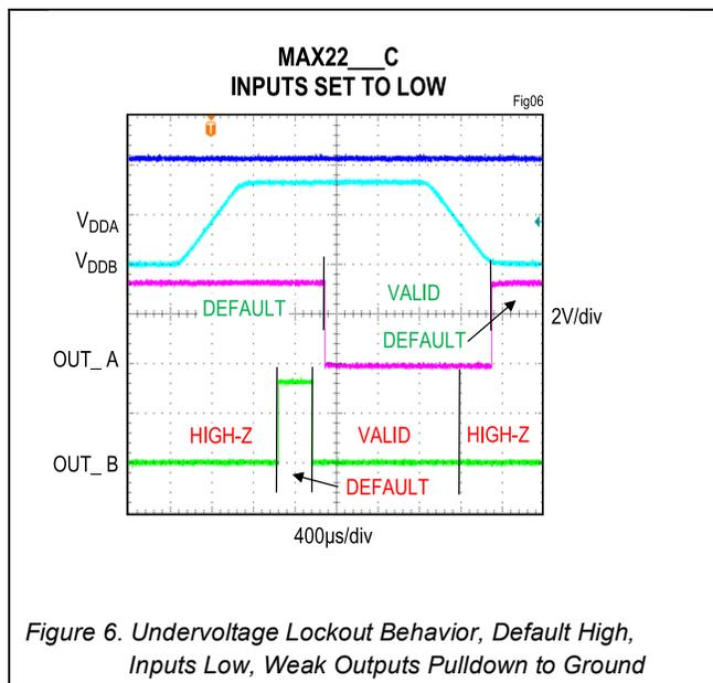
Figure 6. Undervoltage Lockout Behavior, Default High, Inputs Low, Weak Outputs Pulldown to Ground
