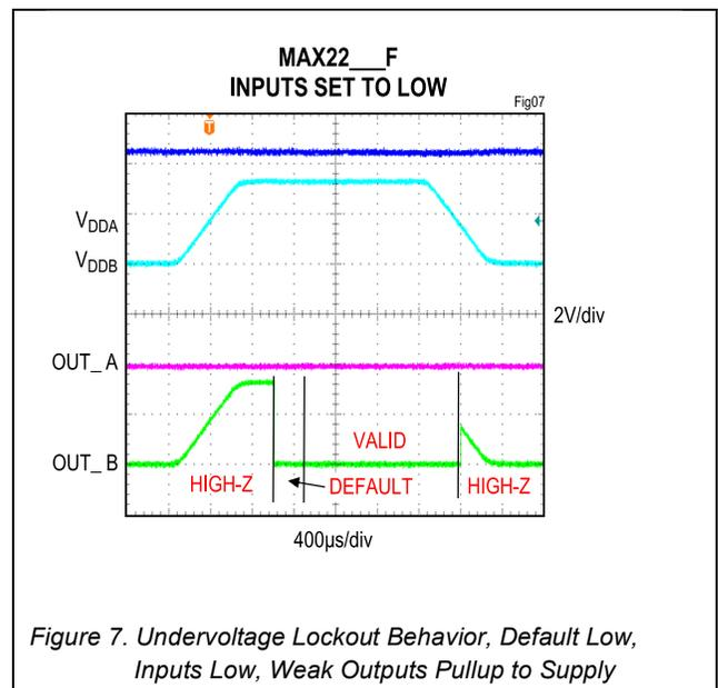
Figure 7. Undervoltage Lockout Behavior, Default Low, Inputs Low, Weak Outputs Pullup to Supply
