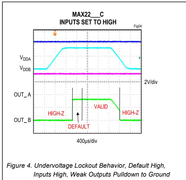
Figure 4. Undervoltage Lockout Behavior, Default High, Inputs High, Weak Outputs Pulldown to Ground
