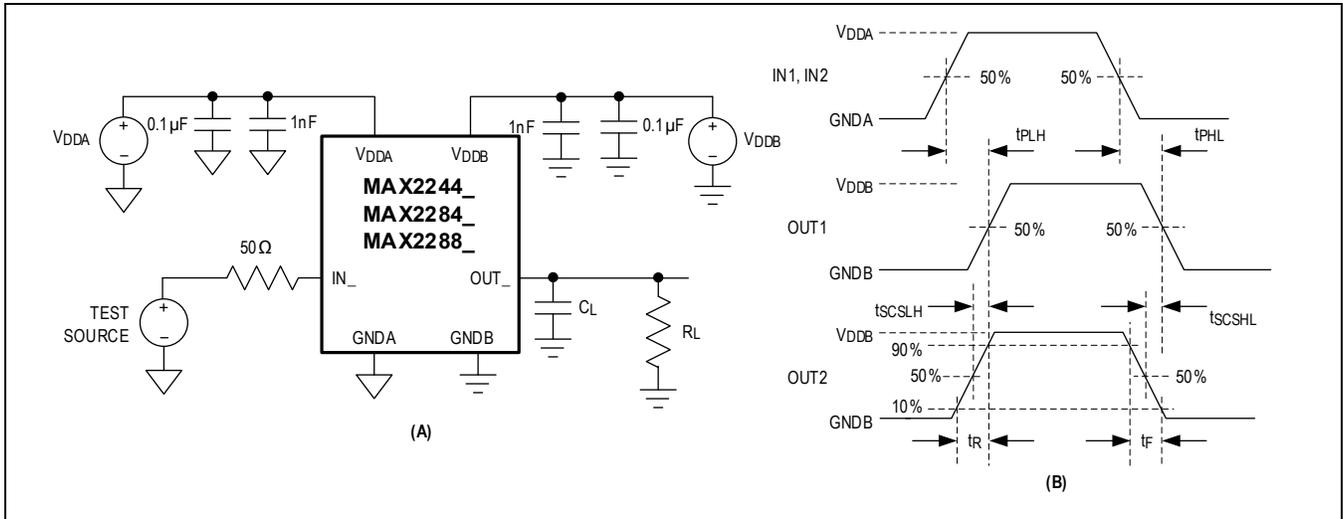
Figure 1. Test Circuit (A) and Timing Diagrams (B)
