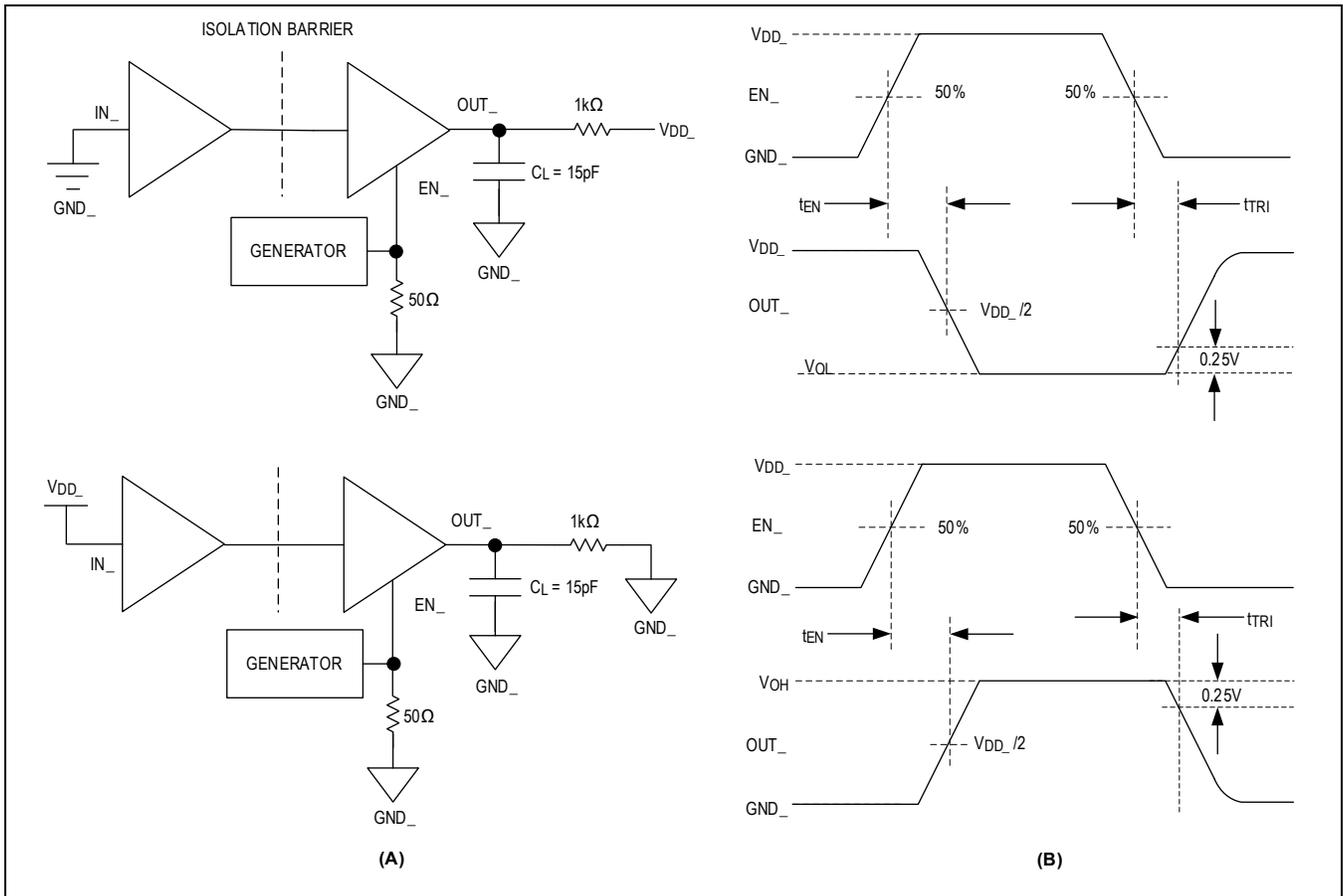
Figure 2. Enable to Output Timing Diagrams ( $t_{EN}$ ,  $t_{TRI}$ )
