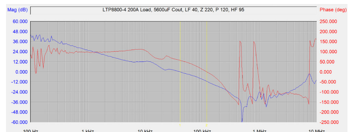
Figure 3. Measured Bode Plot of the LTP8800-4A
