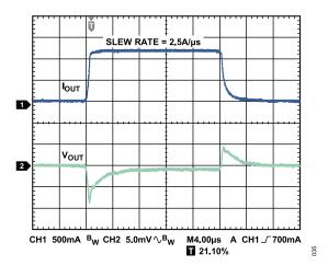
Figure 32. Load Transient Response,  $I_{LOAD}$  = 100 mA to 1.2 A,  $V_{OUT}$  = 3.3 V,  $V_{IN}$  = 4.0 V, Channel 1 =  $I_{OUT}$ , Channel 2 =  $V_{OUT}$
