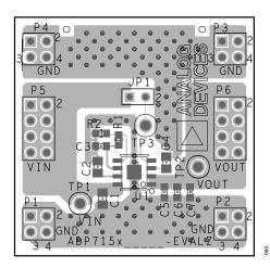
Figure 62. Sample 8-Lead SOIC PCB Layout
