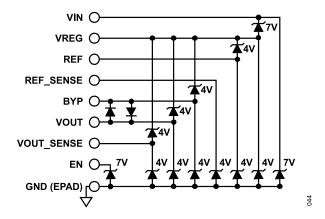
Figure 41. Simplified ESD Protection Block Diagram
