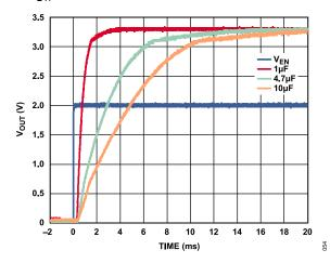
Figure 51. Typical Start-Up Behavior with  $C_{BYP} = 1 \mu F$  to 10  $\mu F$
