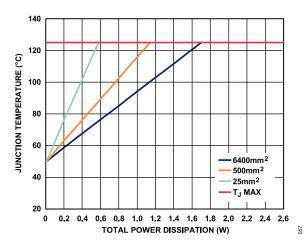
Figure 54. Junction Temperature vs. Total Power Dissipation for the 10-Lead LFCSP,  $T_{\Delta}$  = 50°C
