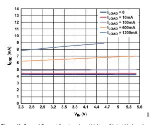
Figure 19. Ground Current ( $I_{GND}$ ) vs. Input Voltage ( $V_{IN}$ ) at Various Loads,  $V_{OUT}$  = 1.8 V
