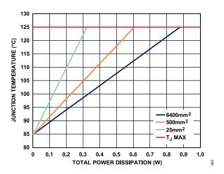
Figure 58. Junction Temperature vs. Total Power Dissipation for the 8-Lead SOIC,  $T_A$  = 85°C
