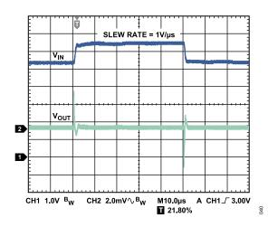
Figure 37. Line Transient Response, 1 V Input Step,  $I_{LOAD}$  = 1.2 A,  $V_{OUT}$  = 1.8 V,  $V_{IN}$  = 2.5 V, Channel 1=  $V_{IN}$ , Channel 2 =  $V_{OUT}$
