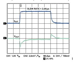
Figure 42. Output Transient Response,  $V_{OUT}$  = 3.3 V,  $C_{OUT}$  = 10  $\mu$ F, Channel 1 = Load Current, Channel 2 =  $V_{OUT}$
