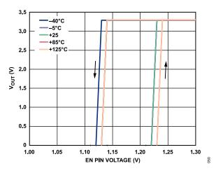
Figure 47. Typical V<sub>OUT</sub> Response to EN Pin Operation
