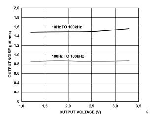
Figure 28. RMS Output Noise vs. Output Voltage
