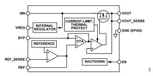
Figure 40. Simplified Internal Block Diagram
