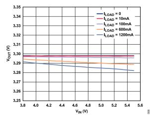
Figure 7. Output Voltage ( $V_{OUT}$ ) vs. Input Voltage ( $V_{IN}$ ) at Various Loads,  $V_{OUT}$ = 3.3 V
