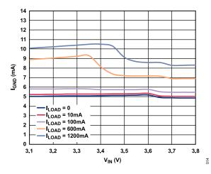
Figure 13. Ground Current ( $I_{\rm GND}$ ) vs. Input Voltage ( $V_{\rm IN}$ ) at Various Loads in Dropout,  $V_{\rm OUT}$  = 3.3 V
