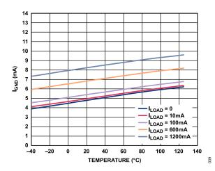
Figure 8. Ground Current ( $I_{GND}$ ) vs. Temperature at Various Loads,  $V_{OUT}$  = 3.3 V
