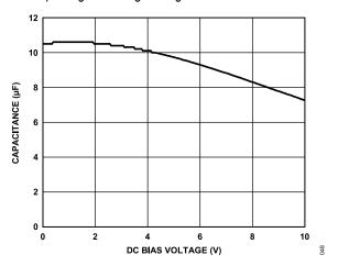
Figure 45. Capacitance vs. DC Bias Voltage
