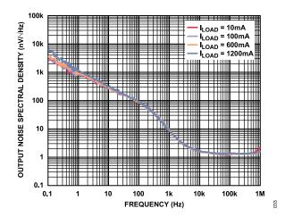
Figure 30. Output Noise Spectral Density vs. Frequency at Various Loads, 0.1 Hz to 1 MHz
