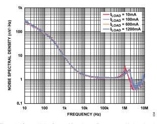
Figure 31. Output Noise Spectral Density vs. Frequency at Various Loads, 10 Hz to 10 MHz
