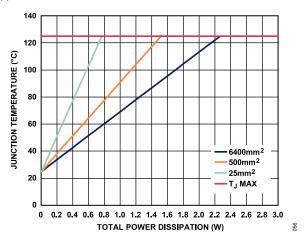
Figure 53. Junction Temperature vs. Total Power Dissipation for the 10-Lead LFCSP,  $T_{\Delta}$  = 25°C
