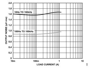
Figure 27. RMS Output Noise vs. Load Current
