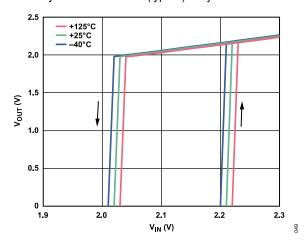
Figure 46. Typical UVLO Behavior at Various Temperatures, V<sub>OUT</sub> = 3.3 V
