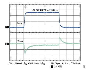
Figure 34. Load Transient Response,  $I_{LOAD}$  = 100 mA to 1.2 A,  $V_{OUT}$  = 1.8 V,  $V_{IN}$  = 2.5 V, Channel 1 =  $I_{OUT}$ , Channel 2 =  $V_{OUT}$
