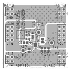
Figure 61. Sample 10-Lead LFCSP PCB Layout
