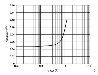
Figure 11. Dropout Voltage ( $V_{DROPOUT}$ ) vs. Load Current ( $I_{LOAD}$ ),  $V_{OUT}$  = 3.3 V
