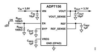
Figure 50. Typical EN Pin Voltage Divider
