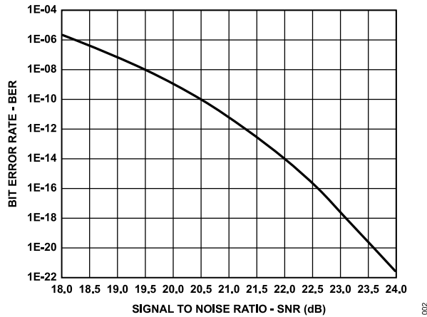
Figure 16. Statistical Relation Between SNR and BER in 10BASE-T1L
