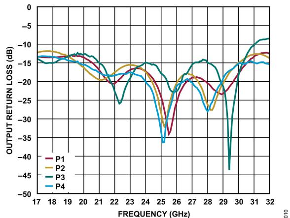
Figure 10. Output Return Loss vs. Frequency (P1, P2, P3, and P4)
