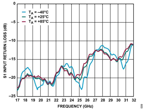
Figure 9. S1 Input Return Loss vs. Frequency over Temperature
