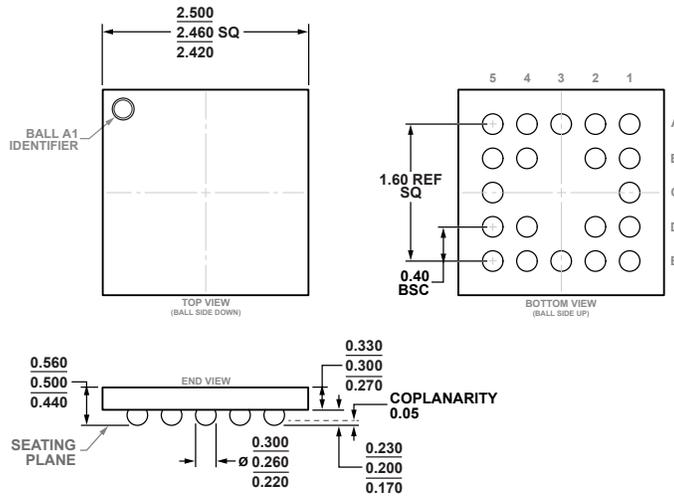
Figure 15. 20-Ball Wafer Level Chip Scale Package [WLCSP] (CB-20-17)
