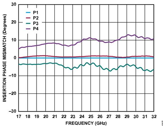
Figure 7. Insertion Phase Mismatch vs. Frequency, All Paths Normalized to P1
