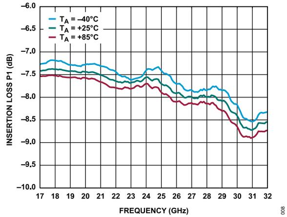
Figure 8. Insertion Loss P1 vs. Frequency over Temperature
