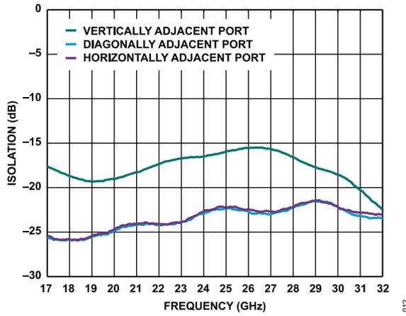
Figure 12. Isolation vs. Frequency
