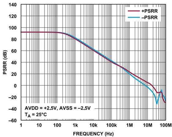
Figure 56. PSRR vs. Frequency, AVDD = +2.5 V, AVSS = -2.5 V
