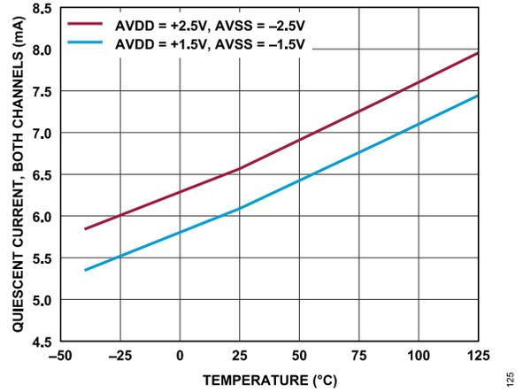
Figure 75. AVDD Quiescent Current, Both Channels vs. Temperature
