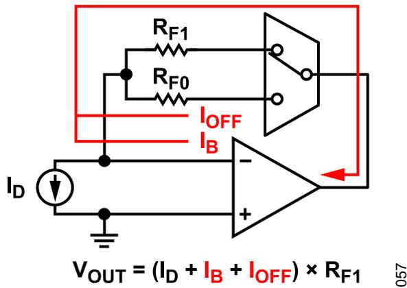
Figure 79. Error Currents in Switched Gain Transimpedance Amplifier
