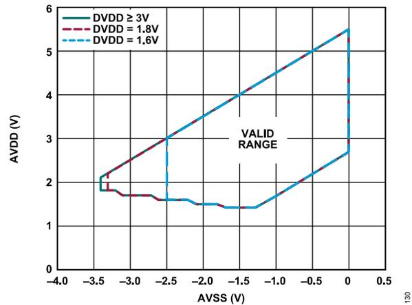
Figure 77. Valid Operating Range for AVSS Below DVSS, DVSS = 0 V
