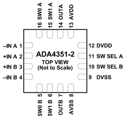
Figure 5. Pin Configuration
