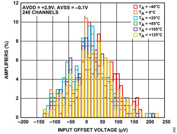
Figure 15. Offset Voltage Distribution, AVDD = +2.9 V, AVSS = -0.1 V
