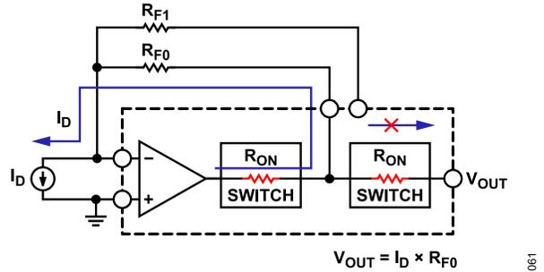
Figure 83. Switched Gain Transimpedance Amplifier with Kelvin Switching
