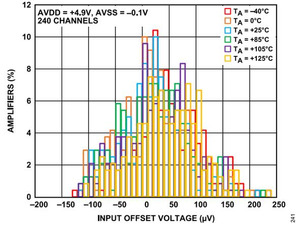
Figure 9. Offset Voltage Distribution, AVDD = +4.9 V, AVSS = -0.1 V
