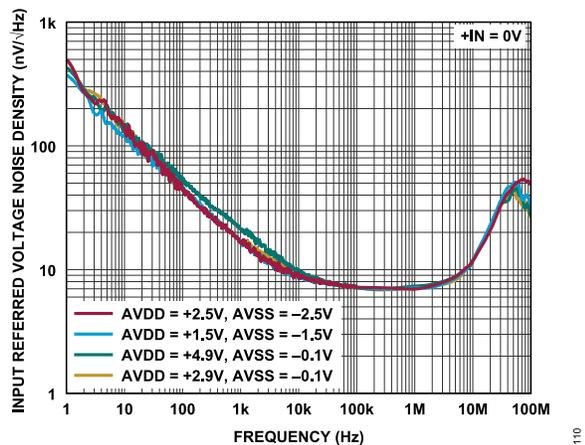
Figure 50. Input Referred Voltage Noise Density vs. Frequency
