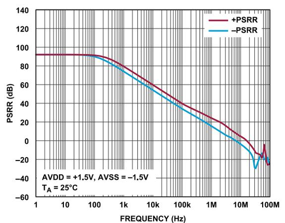
Figure 59. PSRR vs. Frequency, AVDD = +1.5 V, AVSS = -1.5 V
