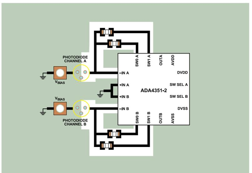
Figure 98. Example PCB Layout for Low Surface Leakage
