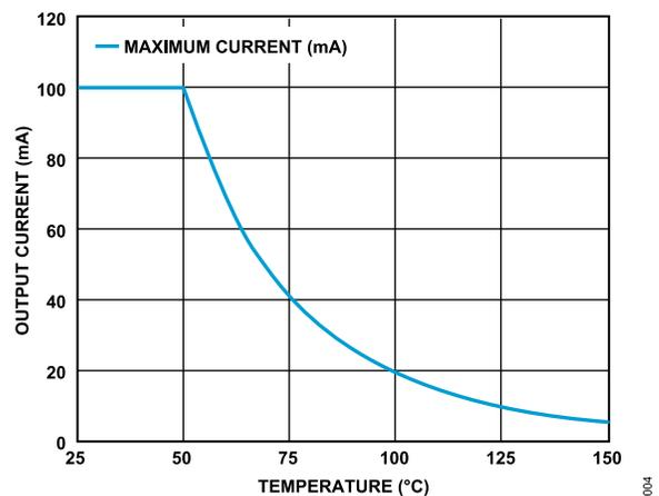
Figure 4. Maximum Output Current Derating Curve vs. Temperature
