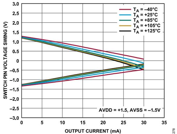
Figure 41. Switch Pin Voltage Swing vs. Output Current at Various Temperatures,  $R_F = 200\ \Omega$ , AVDD = +1.5 V, AVSS = -1.5 V
