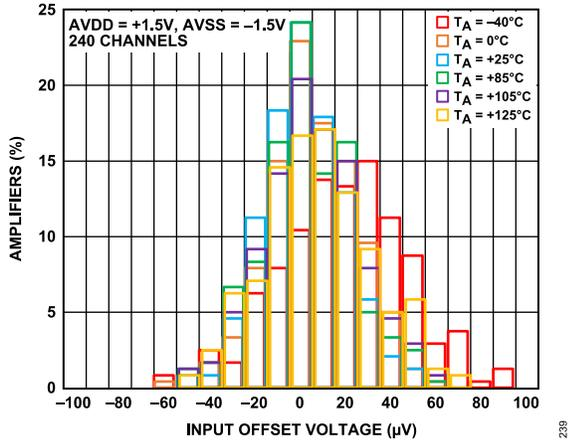
Figure 12. Offset Voltage Distribution, AVDD = +1.5 V, AVSS = -1.5 V
