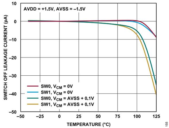
Figure 34. Switch Off Leakage Current vs. Temperature for Various SW0 and SW1 V<sub>CM</sub> Values, AVDD = +1.5 V, AVSS = -1.5 V
