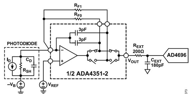
Figure 94. Typical Single-Supply Application Using the AD4696
