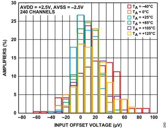
Figure 6. Offset Voltage Distribution, AVDD = +2.5 V, AVSS = -2.5 V
