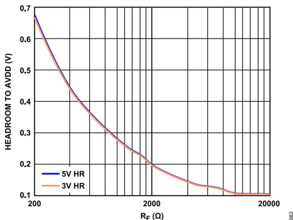
Figure 84. Output Headroom (HR) to AVDD vs.  $R_F$
