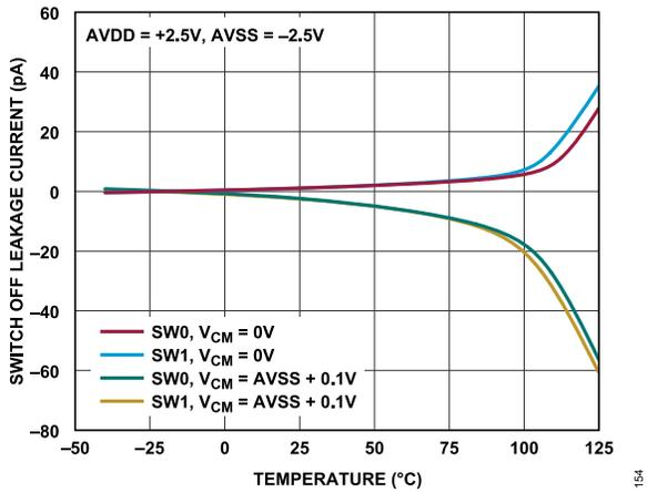
Figure 31. Switch Off Leakage Current vs. Temperature for Various SW0 and SW1 V<sub>CM</sub> Values, AVDD = +2.5 V, AVSS = -2.5 V
