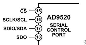
Figure 50. Serial Control Port
