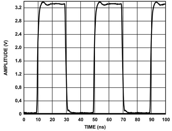
Figure 15. CMOS Output with 10 pF Load at 25 MHz
