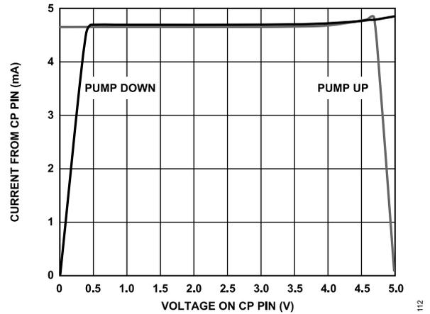
Figure 9. Charge Pump Characteristics at  $CP_V = 5.0 V$
