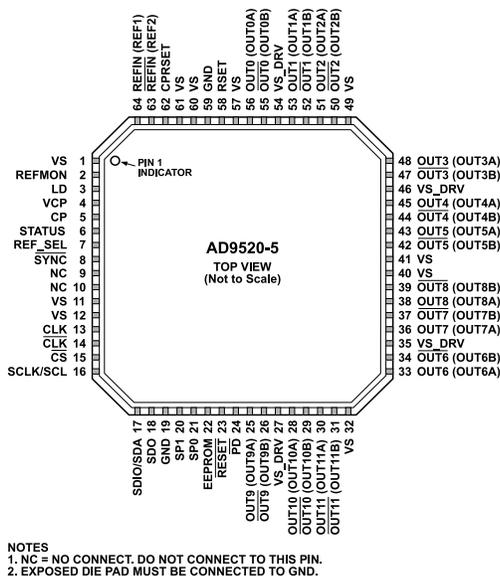
Figure 5. Pin Configuration
