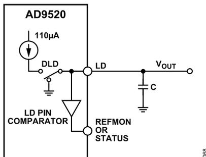
Figure 33. Current Source Digital Lock Detect
