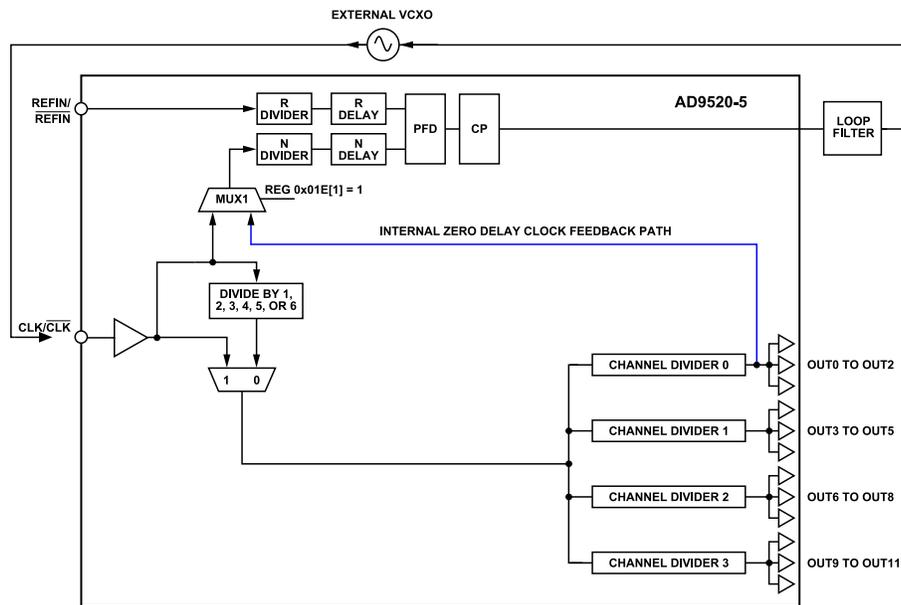
Figure 37. Zero Delay Function
