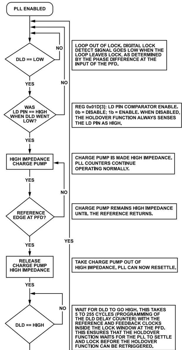
Figure 35. Flowchart of Automatic/Internal Holdover Mode
