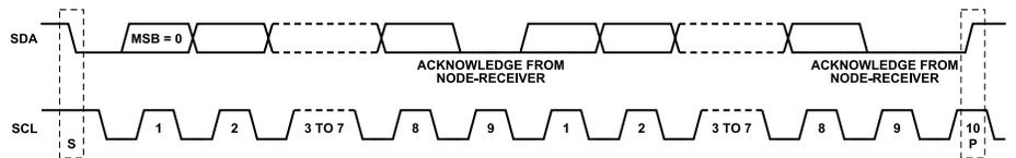
Figure 47. Data Transfer Process (Main Write Mode, 2-Byte Transfer Used for Illustration)
