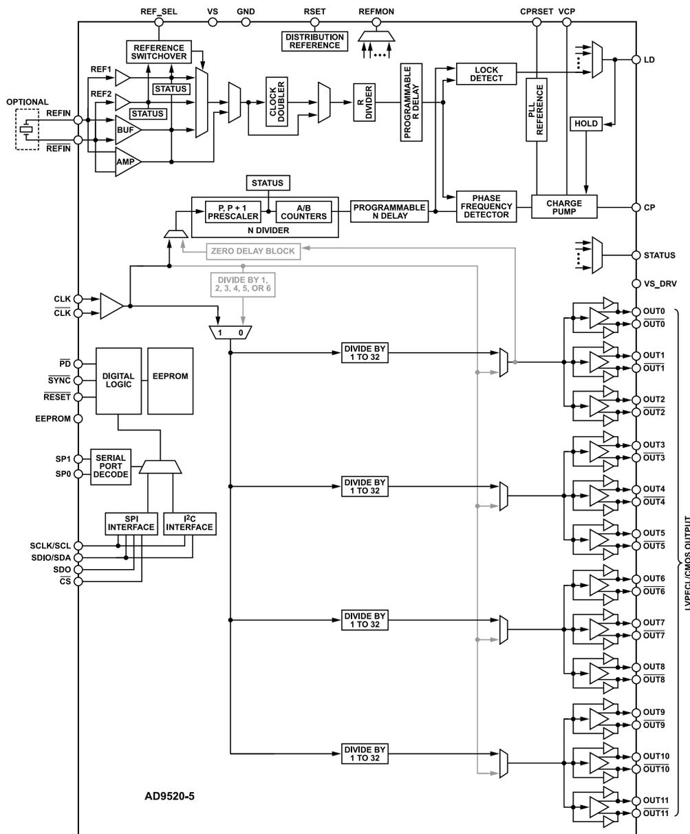
Figure 27. Clock Distribution or External VCO < 1600 MHz (Mode 1)
