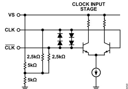
Figure 34. CLK Equivalent Input Circuit
