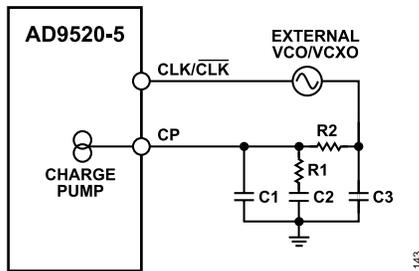
Figure 30. Example of External Loop Filter for PLL
