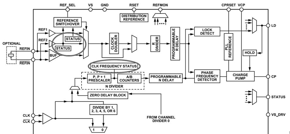
Figure 36. Reference and CLK Frequency Status Monitors
