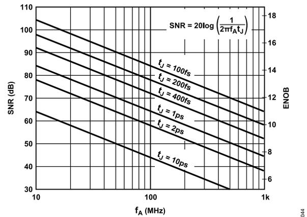
Figure 58. SNR and ENOB vs. Analog Input Frequency
