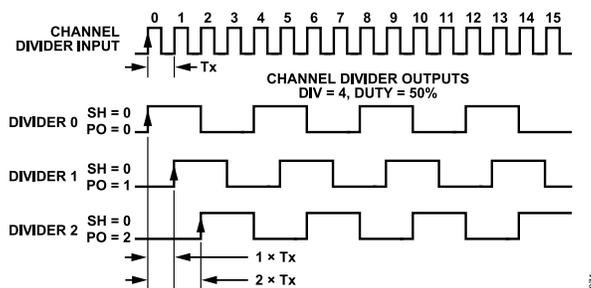
**Figure 39. Effect of Coarse Phase Offset (or Delay)**
