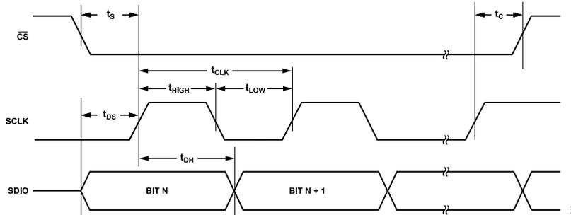
Figure 57. Serial Control Port Timing—Write
