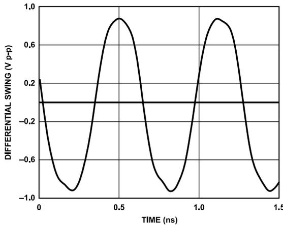
Figure 14. LVPECL Differential Voltage Swing at 1600 MHz
