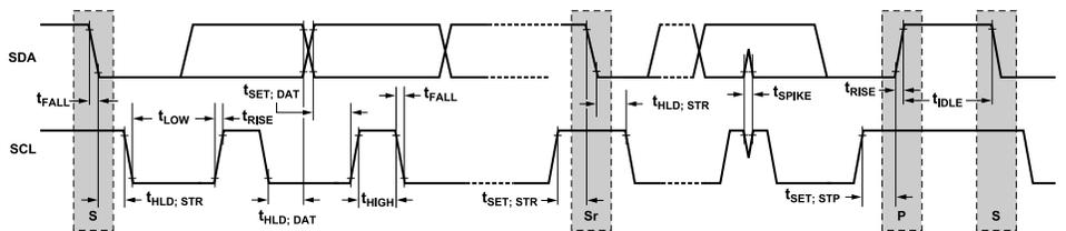
Figure 49. I<sup>2</sup>C Serial Port Timing
