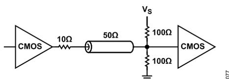
Figure 63. CMOS Output with Far-End Termination
