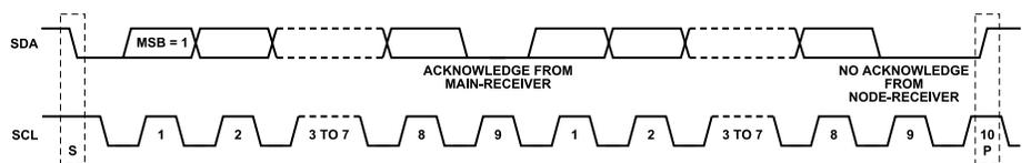
Figure 48. Data Transfer Process (Main Read Mode, 2-Byte Transfer Used for Illustration)
