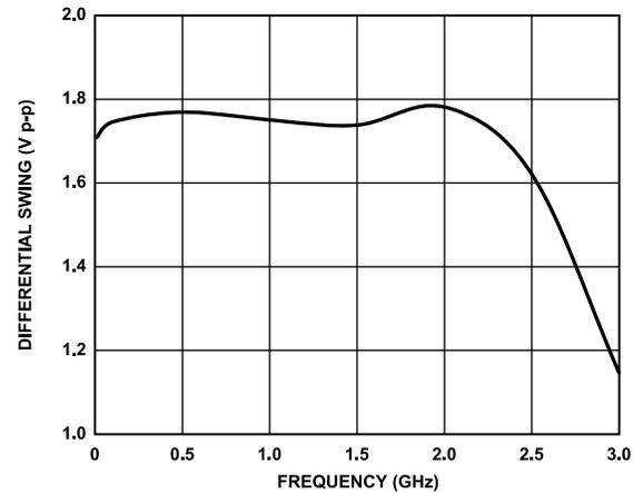
Figure 17. LVPECL Differential Voltage Swing vs. Frequency
