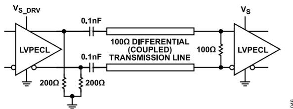
Figure 61. AC-Coupled LVPECL with Parallel Transmission Line
