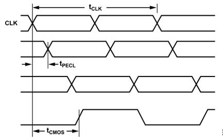
Figure 3. CLK/CLK to Clock Output Timing, DIV = 1
