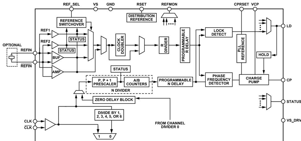
Figure 29. PLL Functional Block Diagram
