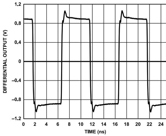
Figure 13. LVPECL Output (Differential) at 100 MHz
