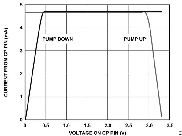
Figure 8. Charge Pump Characteristics at  $CP_V = 3.3 V$
