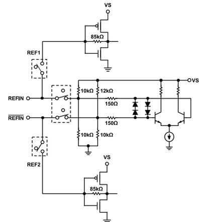
Figure 31. REF<sub>IN</sub> Equivalent Circuit for Non-XTAL Mode
