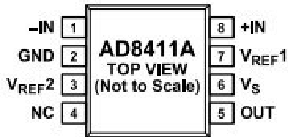
Figure 4. 8-Lead MSOP and 8-Lead SOIC Pin Configuration
