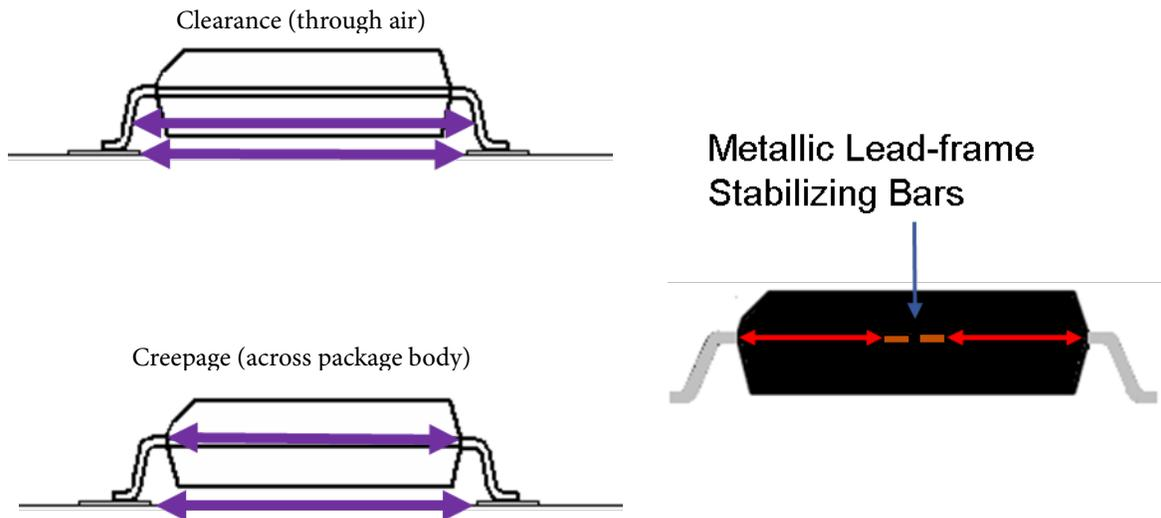
Figure 2. Creepage and Clearance
