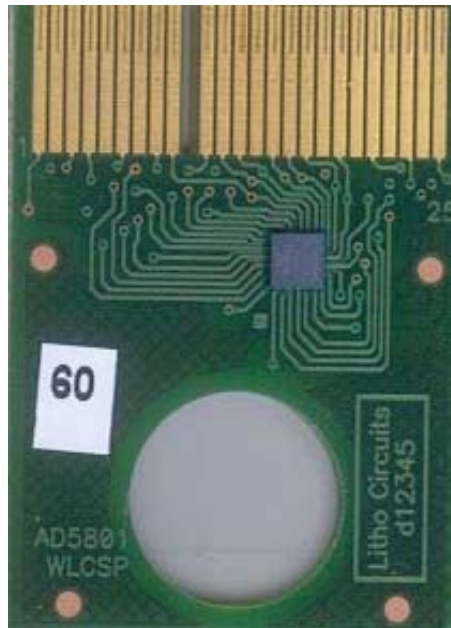
Figure 13. Example of MicroCSP Reliability Test Boards
