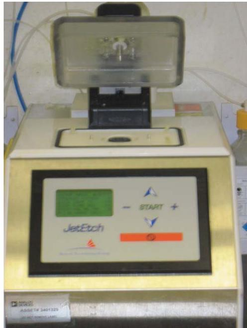
Figure 124. JetEtch Decapsulation Machine
