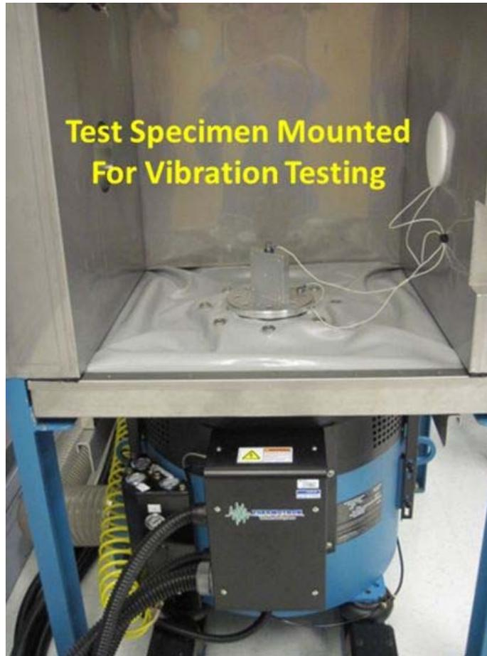
Figure 95. Thermotron DSX-2250 Temperature/Vibration System
