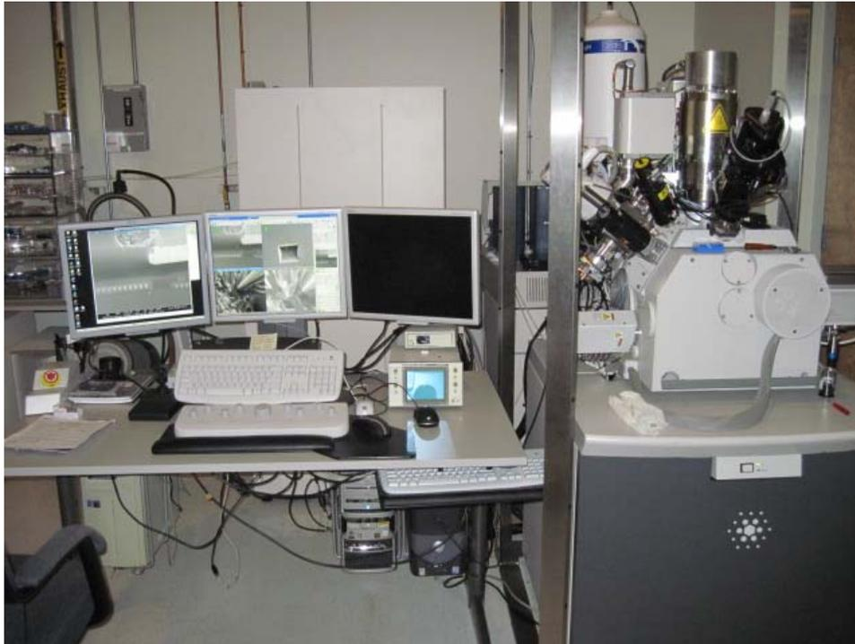
Figure 134. Scanning Electron Microscopy Station
