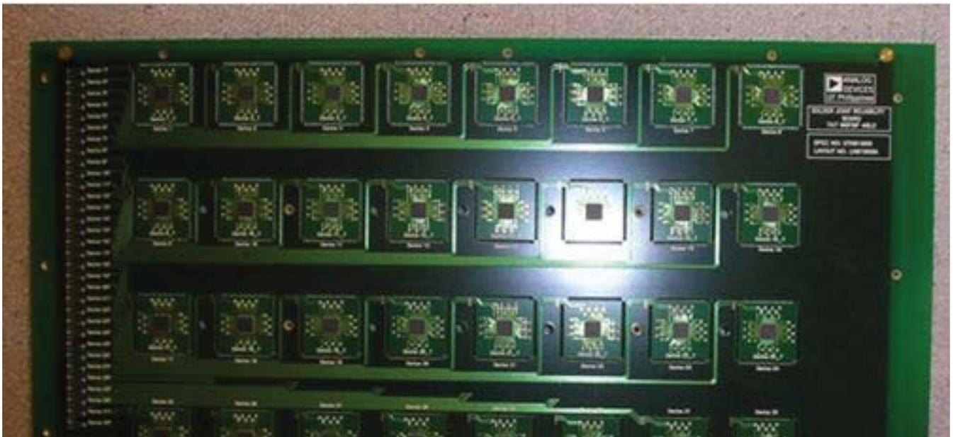
Figure 87. SJR Test Board
