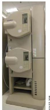
Figure 9. Bank of Autoclave Chambers
