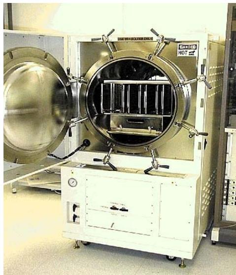
Figure 11. Typical HAST Test System
