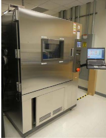
Figure 10. Temperature and Humidity Chamber
