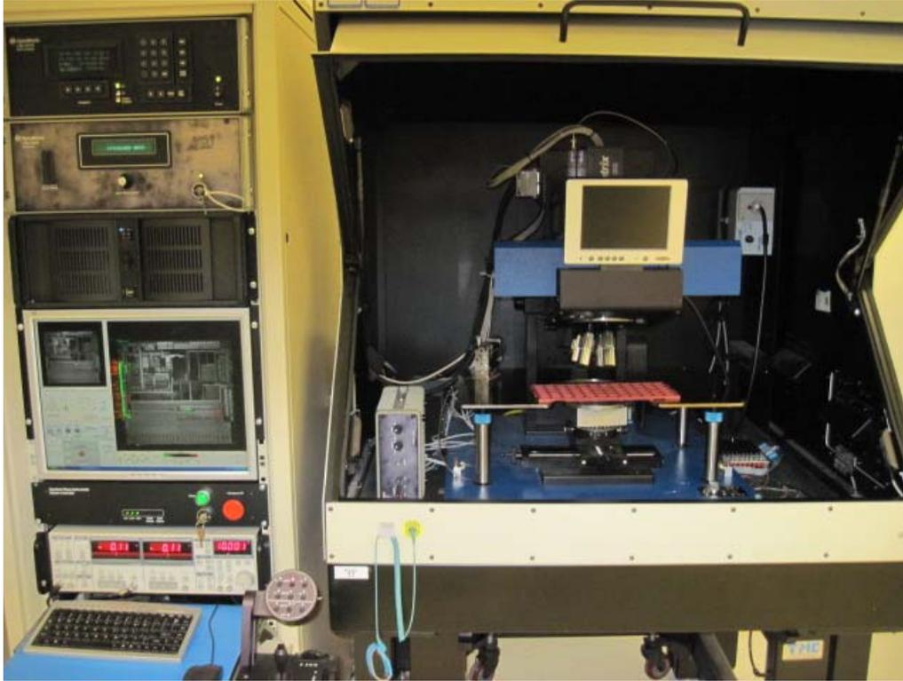
Figure 130. Electrical Microprobing Station
