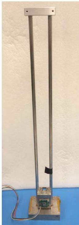
Figure 100. Guillotine Powered Mechanical Shock Test Fixture
