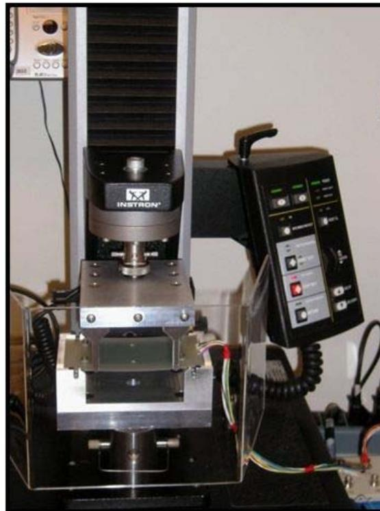
Figure 93. Instron 4455A Bend Tester
