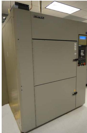
Figure 12. Typical Temperature Cycle Test Chambers
