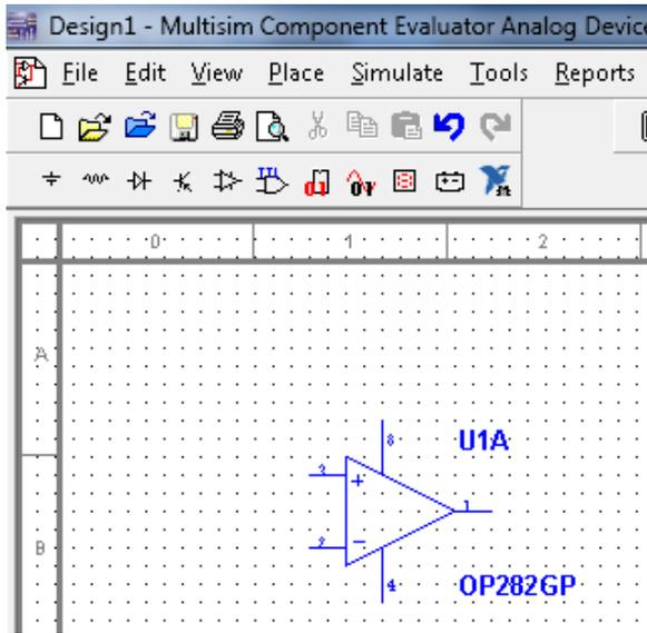
Figure 4. A Single Op Amp Ready for More Connections
