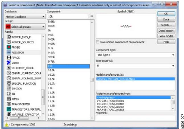
Figure 7. Selecting Resistor Values
