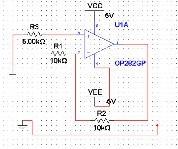
Figure 8. All Resistors Placed, but Some Connections Missing
