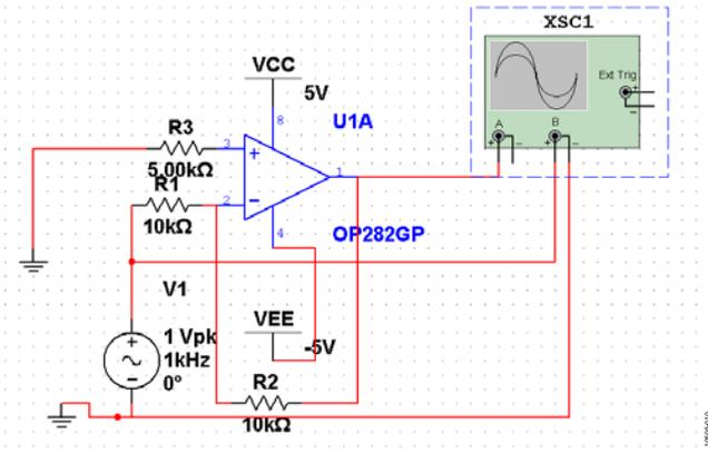
Figure 10. Connecting the Input Source and an Oscilloscope to the Output
