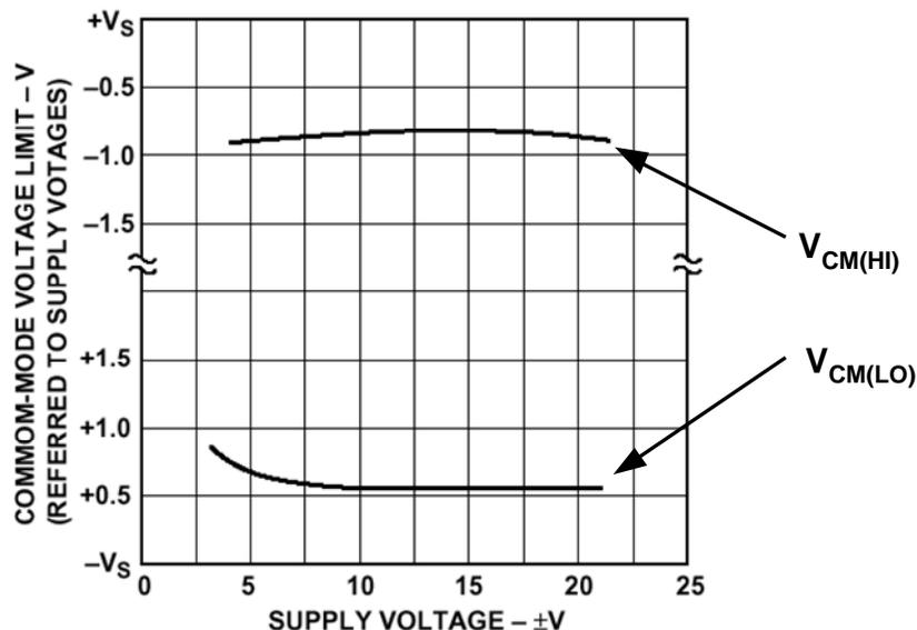
**Figure 2: A Graphical Display of Op Amp Input Common-Mode Range**
