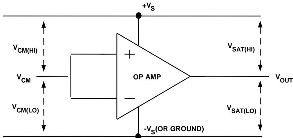
**Figure 1: Op Amp Input and Output Common-Mode Ranges**
