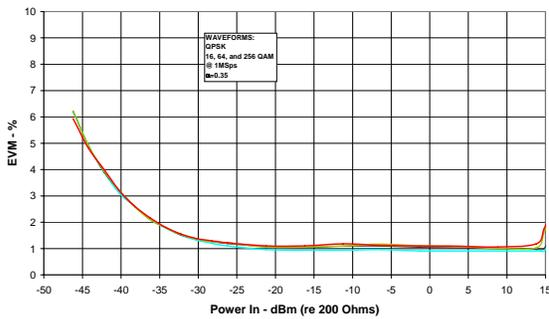
Figure 7. EVM versus input power for 16, 64, and 256QAM.
