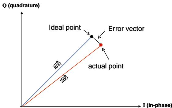
Figure 1. IQ signal space illustrating reference vector,  $R(k)$ , and measurement vector,  $Z(k)$ .
