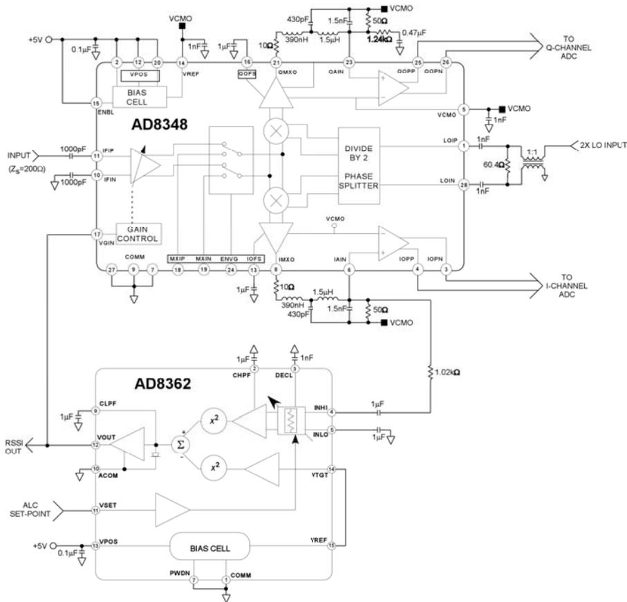
Figure 4. The AD8348 IQ Demodulator in combination with the AD8362 TruPwr™ Detector can be configured to provide highly accurate automatic level control IF-to-baseband receiver subsystem.
