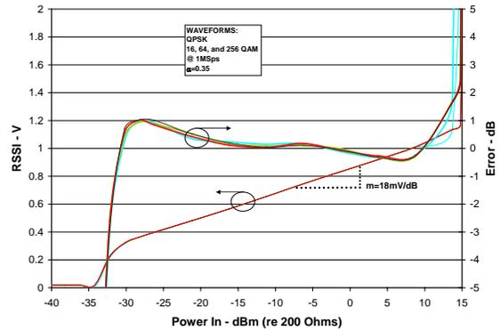
Figure 8. By understanding the EVM versus input power relationships, an rms-accurate RSSI measurement can be used to predict receiver performance.
