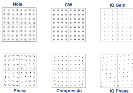
Figure 3. A variety of possible signal impairments. By recognizing the tell-tale signs of different signal impairments, receiver problems can be more easily isolated and debug simplified.
