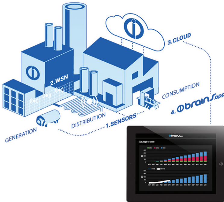
Figure 3. Driving Change—Software Analytics, Such as the Brains.App Software from IntelliSense.io, Use the Data from Industrial Wireless Sensor Networks to Streamline Plant Operations, Optimize Yield and Improve Safety
