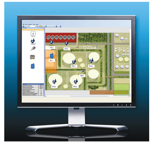
Figure 2. Network Visibility—Network Management Software Provides Critical Visibility to the Health of the Wireless Network Such as in This SNAP-ON Software Utility from Emerson Process Management
