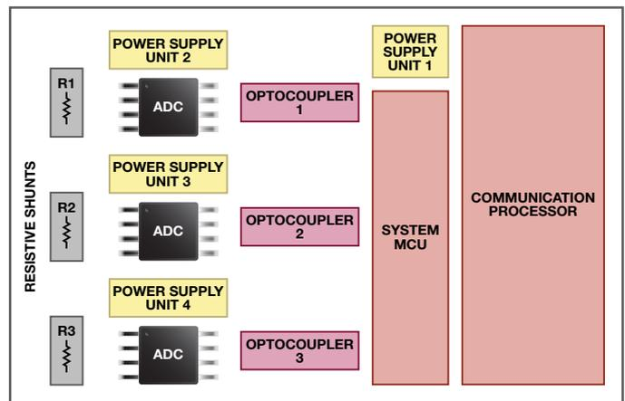
Figure 4. Polyphase smart meter: optocouplers provide isolation.
