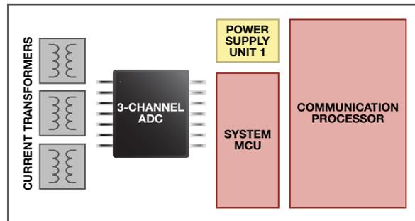
Figure 3. Polyphase smart meter: current transformers provide isolation.
