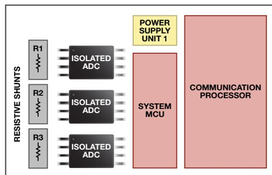
Figure 5. Polyphase smart meter: isolated ADCs provide isolation.
