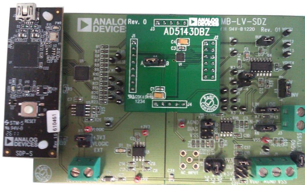
Figure 1. Digital Picture of Evaluation Board with Low Voltage DigiPOT Motherboard and System Demonstration Platform
