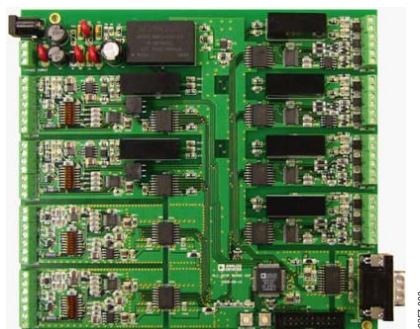
Figure 2. PLC Demo Board
