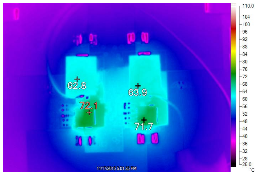
Figure 6. Thermal Picture of DC2394A, V_{IN} = 12V , V_{OUT0} = V_{OUT1} = 1.0V , I_{OUT0} = I_{OUT1} = 30A , F_{SW} = 350kHz , No Airflow, T_A = 25^\circ C
