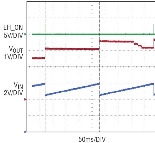
**Figure 2. Midé V25W charging the 18 $\mu$ F input capacitance from 4.48V to 5.92V in 208ms**
