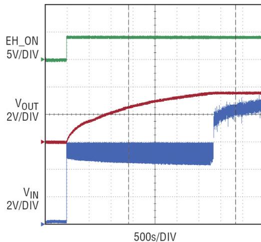
**Figure 3. Midé 25W charging output supercapacitor to 3.6V**
