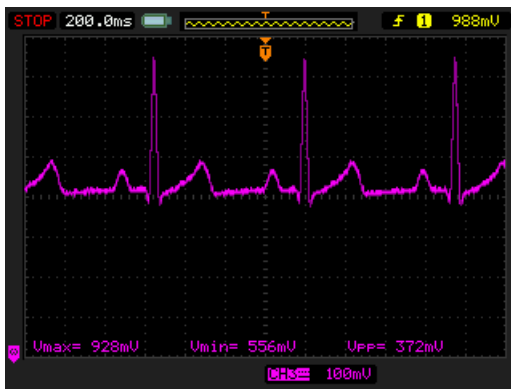
Figure 5. The Monitor's Analog Output Shows Noise Coupled from the Power Line
